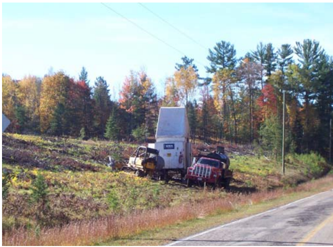
Above: In October 2006, a drilling rig is drilling cores from 1500 feet below ground surface. The cores are analyzed for mineral content and concentration, and for economic viability.
