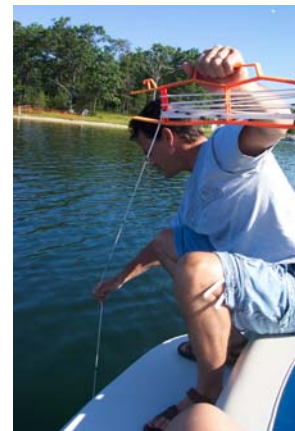
Right: Jim Dixon, a volunteer from Big Star Lake, takes a secchi disk transparency measurement.
