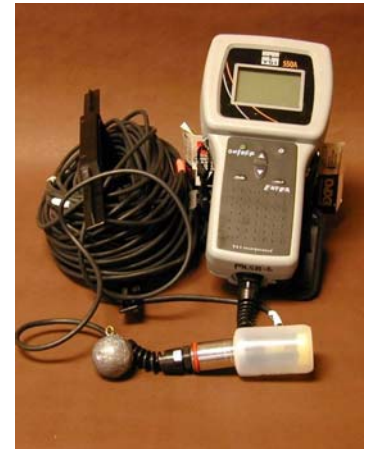
The DO/Temperature meter comes with a very long cable attached to a probe. The probe is lowered from the lake surface to the lake bottom to get DO and temperature profiles (credit: MiCorps staff).
